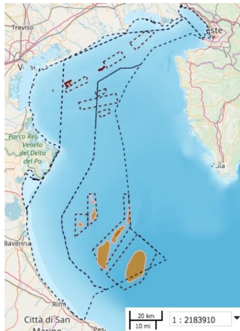
Figure 7: Relict sand deposits of Veneto Region (in brown) and of Emilia Romagna Region (in orange), and potential requests of concessions for extraction (hatched areas)
